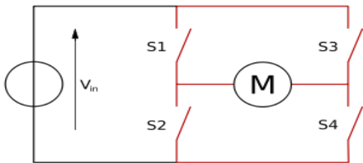
Figure 2: Structure of an H-bridge (highlighted in red)
